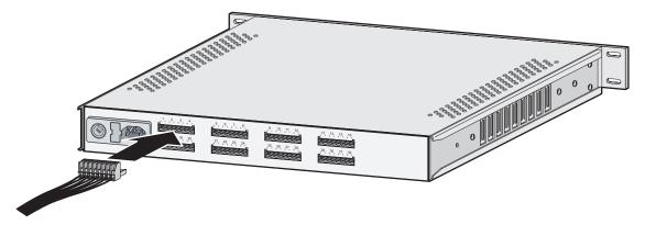
Figure 9. Inserting Terminal Blocks on the Back Panel
